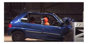
In the above photographs,  $L_1$  is the original length of the car and  $L_2$  is the length of the car after the crash. Thus, the crush distance  $d = L_1 - L_2$ .
